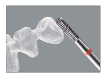
The more thickly milled edges are reduced using a cross-cut tungsten carbide bur. When processing fully anatomical mouldings, the occlusion must be checked.
