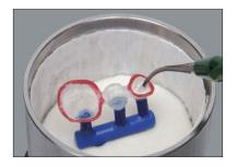
Invest the casting in accordance with the instructions of the investment material manufacturers and place it into the preheating furnace.
