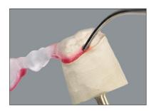
If desired, the ground edges of the moulding can be optimized using casting wax.
