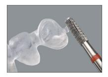
After milling (CAM) the lug is cut off using a fine cross-cut tungsten carbide bur.
