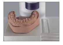
Place the model made from plaster suitable for scanning on the scan holder of the inEos system and carry out the scan process.\*
