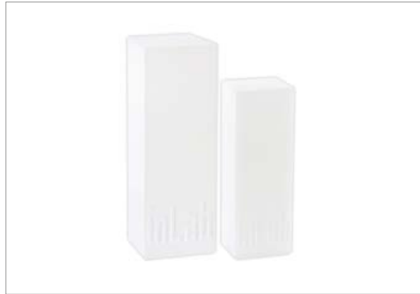
Figure 6: Example of sinter shrinkage of ZrO_2 by approx. 20 %
