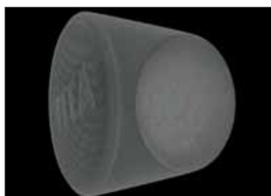
Fig.2: Computer tomographic image (perspective) of a VITA PM 9 press pellet. The structure of the ceramic does not reveal any defect.
