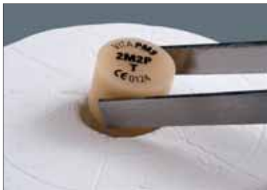
Inserting the VITA PM 9 press pellet
